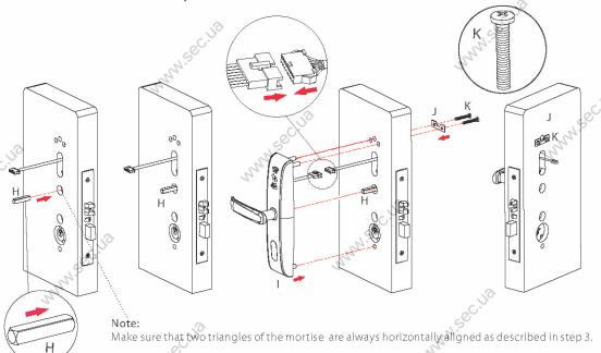
7. Attach the 8x8 spindle (H) and 5x5 spindle (L). Then fix the indoor unit (M)
