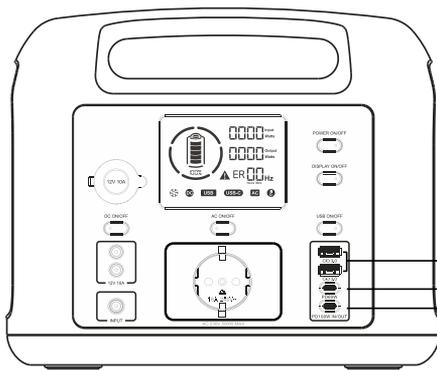
Quick Charger 3.0: 5V $\equiv$ 3A, 3.6V~6V $\equiv$ 3A, 6V~9V $\equiv$ 2A, 9V~12V $\equiv$ 1.5A
