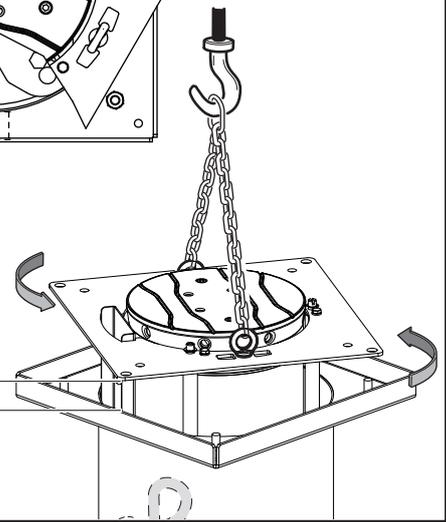
**O** FISSAGGIO DISSUASORE / FASTENING THE BOLLARD / FIXATION DE LA BORNE ESCAMOTABLE
