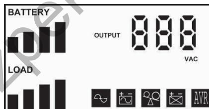
Battery: Battery capacity (25%, 50%, 75%, 100%)
